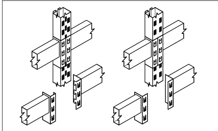
Figure 2: Typical beam-end-connectors of pallet racks.
