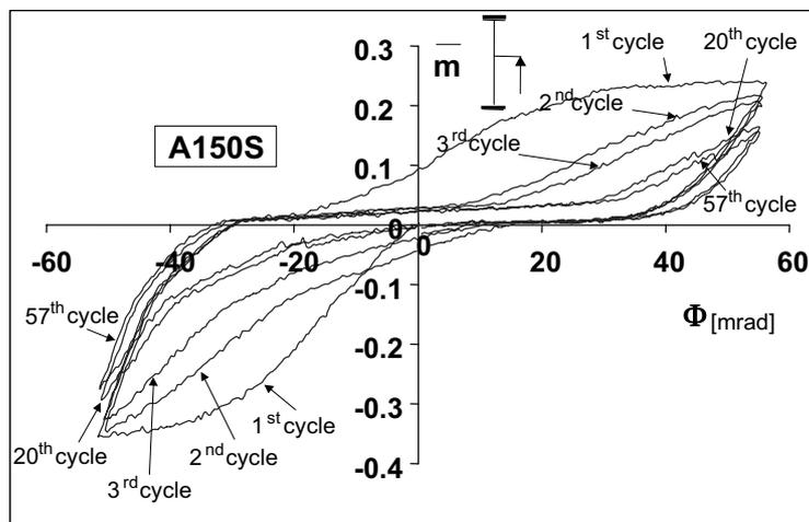
Figure 7: Selected cycles of the  $\bar{m}$ - $\Phi$  curves for A150S joint test.
