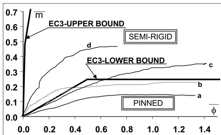
Figure 6: Typical non dimensional moment-rotation joint curves.
