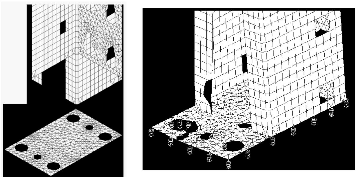
Fig. 4 FEM Simulation of Column Base
