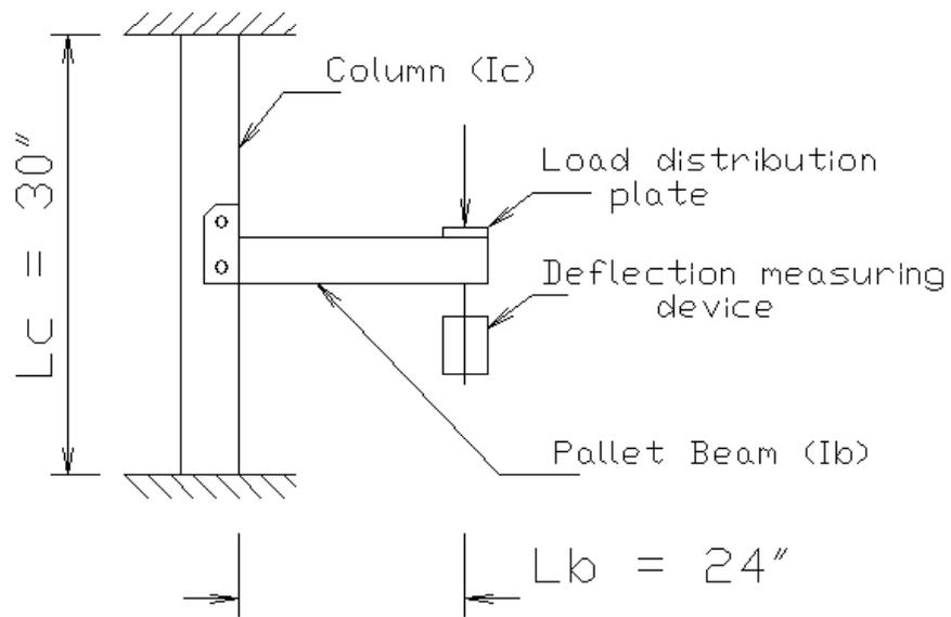
Fig. 1 Cantilever Test Setup
