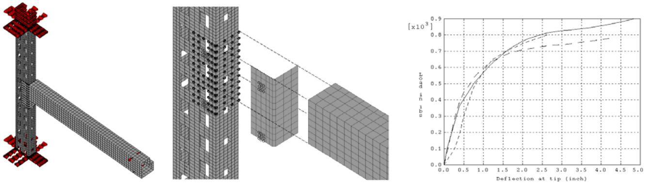
Fig. 3 Simulation of Cantilever tests to get Moment-Rotation Curves. Dashed lines are for two different ways of simulating the joints. One simulation assumes full continuity whereas the other uses contact elements to model the joint more realistically. Solid lines are for physical test results
