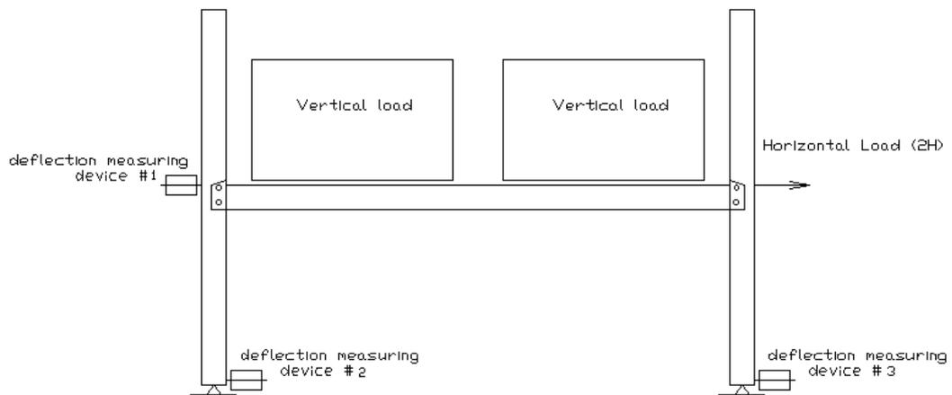
Fig. 2 Portal Test Setup
